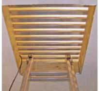
The Loft Hatchway Safety Cover's unique design incorporates folding hollow aluminium slats which hinge to allow access and egress during working. Fixing is by screwing or clamping to the edge of the hatchway while the top side of the slats have anti-slip strips fitted.
