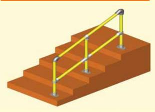
**KwikS3045** is a step section of 48.3mm diameter galvanised steel handrailing 3000mm long with three uprights and flat fix baseplates. The handrail accommodates variable step inclines from 30–45 degrees.
