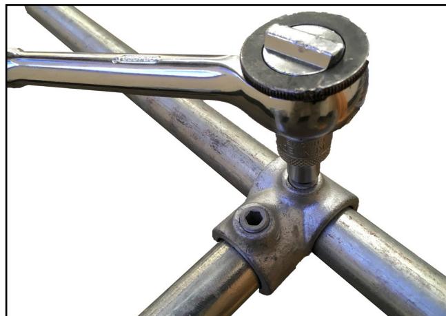
D. Select the 2No. 1925mm lengths of tube and measure and mark the centre of each tube. Slide a (26-5) fitting on to each of the tubes and place the fitting on the centre mark of each tube. Tightening the grub screws using a 1/4" Allen Key. Connect the tubes together and this will now form a large rectangle (frame).
