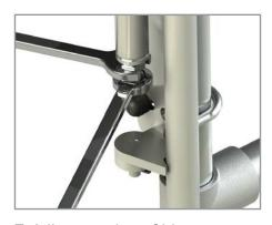
7. Adjust tension of hinge so gate closes fully, and tighten locking nut.
