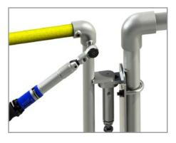
tighten grub screws to 39 Nm.
