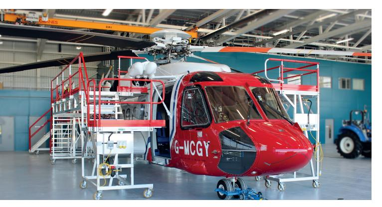
Helicopters often are very awkward or complex shapes, which can be difficult to access. Our platforms are designed to suit tricky layouts and provide a safe solution to working at height. Bearing type castors allow you to effortlessly manoeuvre the units in/out of position, whilst telescopic handrails allow the blades to be rotated and inspected with ease. By using bespoke access equipment, designed specifically for the task in hand, work can be done safely and efficiently.
