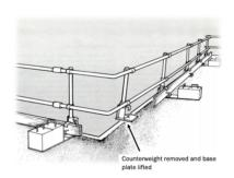
Above: Flat Roof Edge Protection: Proprietary counterweight guardrail system
